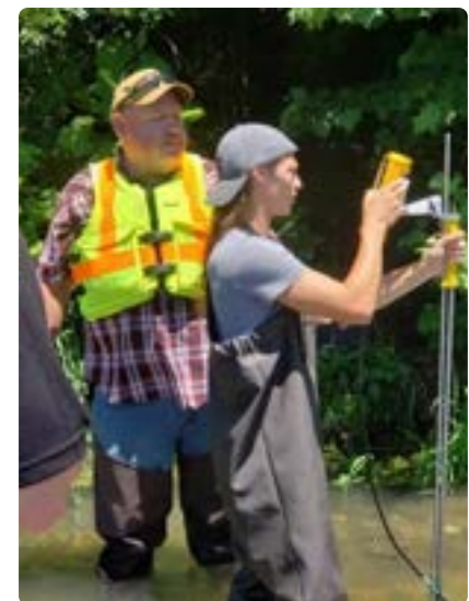
Learning to use a flow meter to measure discharge during a training hosted by Eastern Shawnee Tribe and USGS. 6/5/2024
